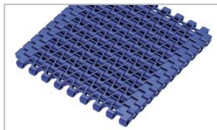
M1280 Flush Grid Pitch 12.85 mm (0.51"), 18% open area
