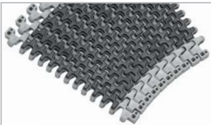
M2544 Radius GripTop Pitch 25.8 mm (1.02"), 38% open area
