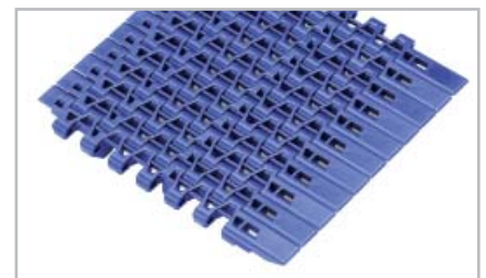
M1280 ActivXchange Pitch 12.85 mm (0.51"), 18% open area
