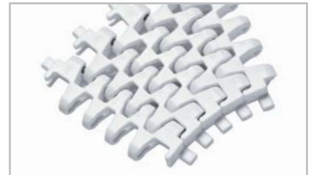
M2544 Tight Radius MTW Pitch 25.8 mm (1.02"), 32% open area
