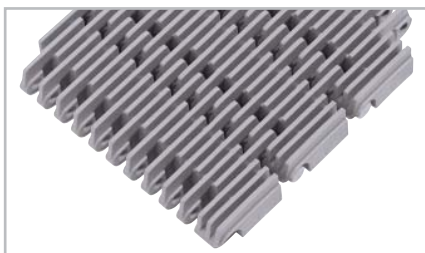
M5131 Raised Rib Pitch 50.8 mm (2"), 36% open area, imperial belt width
