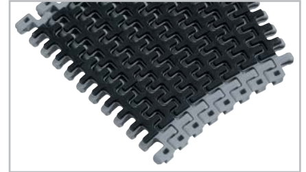
M2540 Radius GripTop Pitch 25.6 mm (1"), 20% open area
